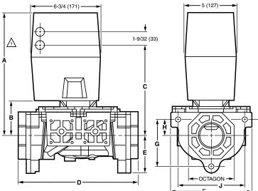
ALLOW 2 IN. (51 MM) CLEARANCE FOR ACTUATOR REMOVAL.
